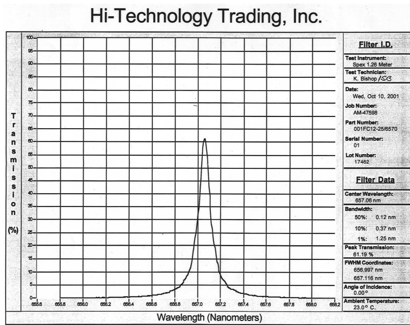
Figure 9: Transmission function of FWHM 0.12 nm filter.
