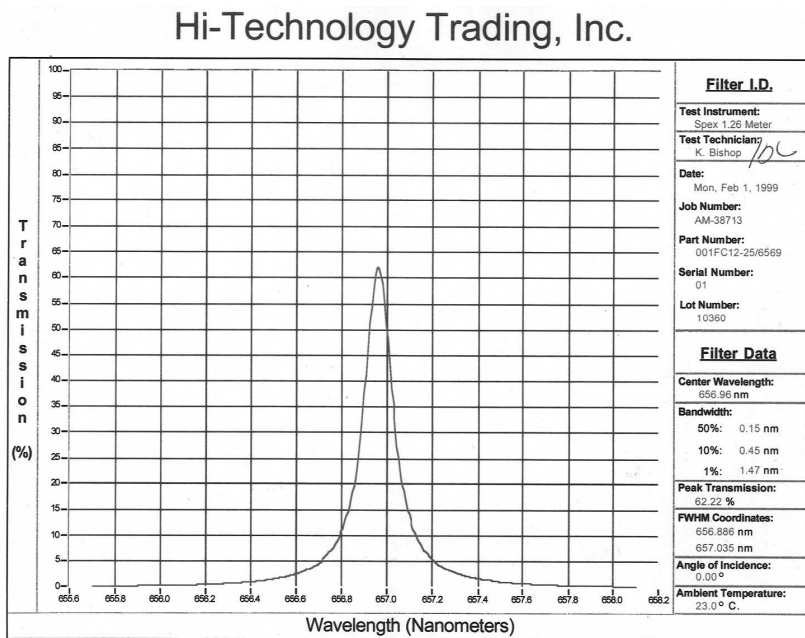
Figure 10: Transmission function of FWHM 0.15 nm filter.
