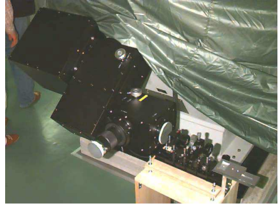
Figure 16: Image sensor mounted at the Coude focus.
