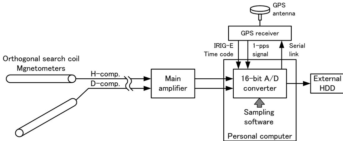
Figure 2.16. Schematic diagram of the ELF observation system.
