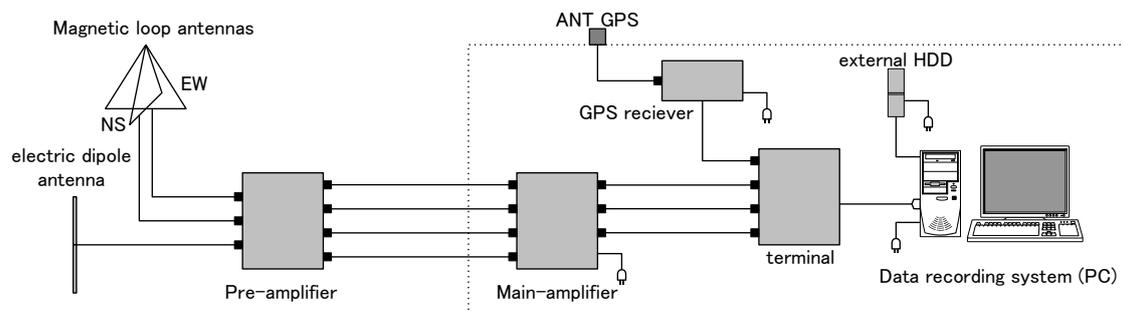
Figure 2.1. Block diagram of the VLF observation system.
