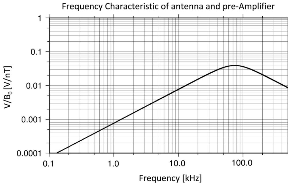
Figure 2.12. Frequency characteristic of gain of magnetic field.
