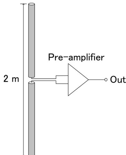
Figure 2.2. Schematic diagram of the antenna and pre-amplifier.
