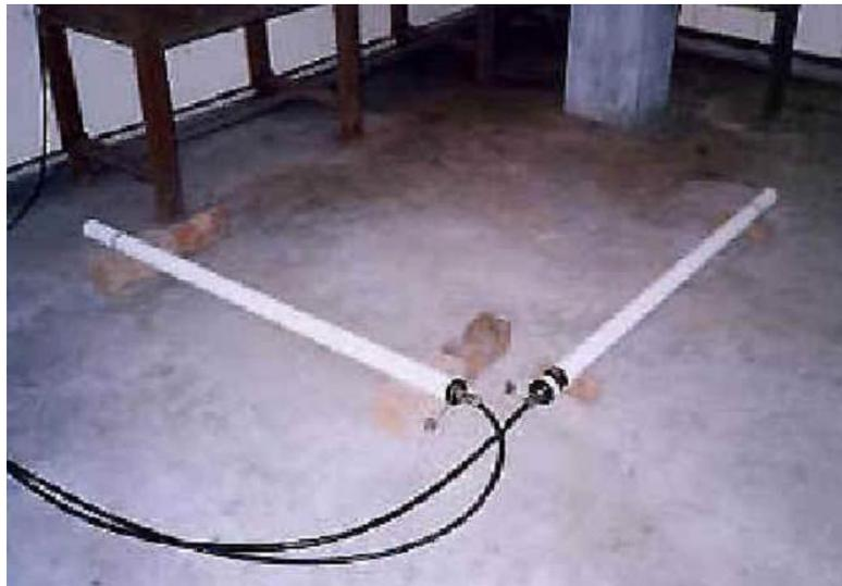
Figure 2.17. View of the magnetic search-coil antenna [Sato, 2004].
